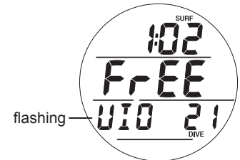
VIOLATION AFTER 1 MIN ON THE SURFACE
